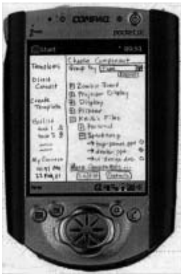
Figure 2: An early, low-fidelity sketch of one of the screens for the Speakeasy Browser. The sketch was drawn inside a photocopy of a Compaq iPAQ PDA, and shows an earlier version of the screen shown in Figure 1
