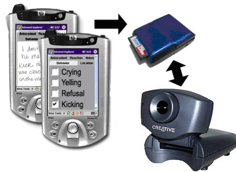
Figure 1: Caregivers take notes on handheld devices using the CareLog application downloaded from the child’s device. CareLog has been augmented to use Bluetooth to discover local experience buffers and request information from them.
